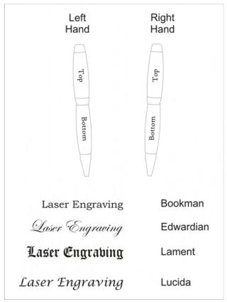
It is always better to engrave before assembly of the pen, so the clip doesn't impede the engraving because of the slight curve involved. We require a sample turned barrel for setup & proof, testing material for laser results, color-fill, font size & placement. It will be centered on barrel unless otherwise requested.
